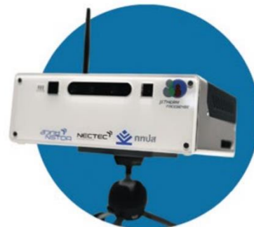
Right: Developed by researchers in Thailand, the temperature-screening system \mu Therm-FaceSense uses a visible camera, a thermal imaging camera, Lidar and facial recognition technology. Photo Credit: Kornrawee Kaewmoon
