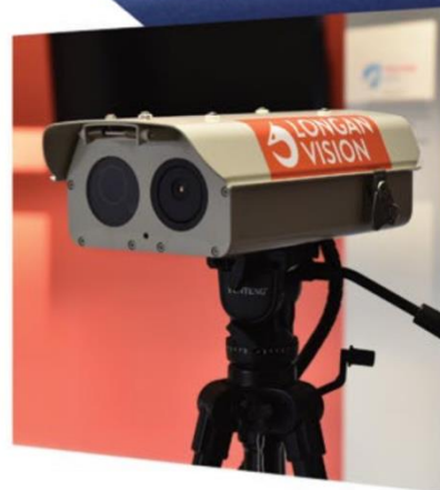
Top: Augmented reality visor with thermal imaging camera Photo Courtesy of Longan Vision Bottom: The Gatekeeper measurement component monitors the calibrated temperature of an area. Photo Courtesy of Longan Vision
