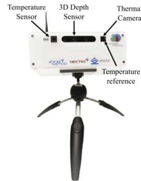
Fig. 2. HTS system embedded with additional electronic temperature sensor, 3-D depth sensor, and temperature reference.
