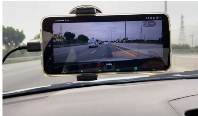
Figure 9 Edge device showing detection by superimposing red rectangle around road irregularity in real time
