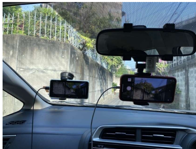
Figure 10 Cross-checking device mounted side-by-side with Edge Device to provide source of truth for reference
