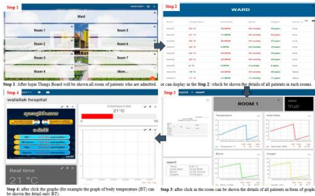
Figure 13. The dashboard screen in the Things Board and steps to display the details of Vital Signals of Patients for nurses and medical professionals monitoring.
