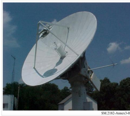
รูปที่ 42 5-metre Scientific-Atlanta azimuth-over-elevation mount full motion antenna
